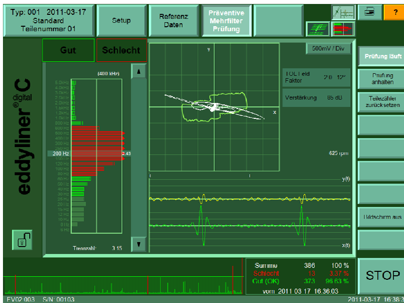
Display of test results as bargraph, y(t)- and x(t)-diagram
