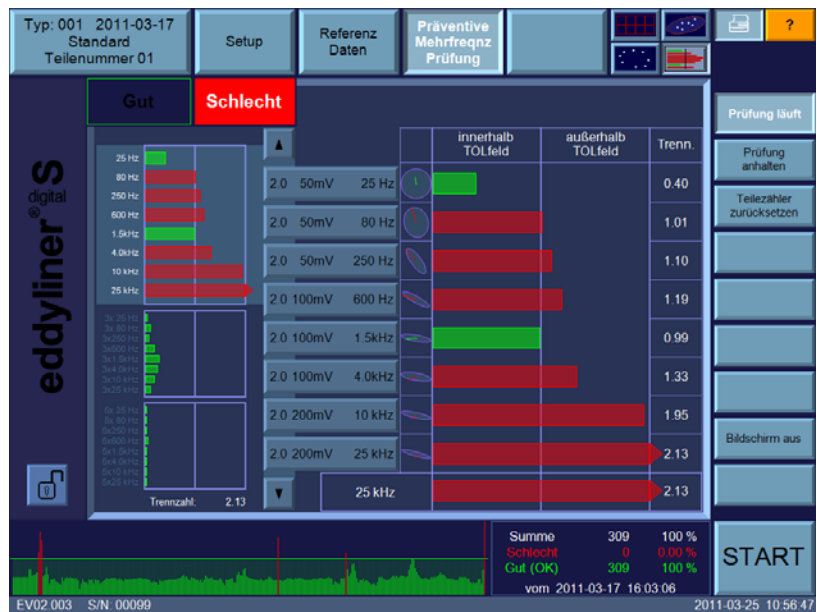
Display with eight tolerance zones as bargraph diagram
